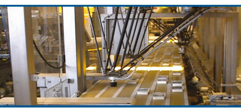
**COMPLEX TASKS** The VARO flexpicker can handle very complex sorting and packaging tasks. It can pick, mix and pack up to 5 different products on the same production line using a high speed scanning system. Furthermore, different types and shapes of trays and cartons can be handled - including glue and tape-free packaging.
